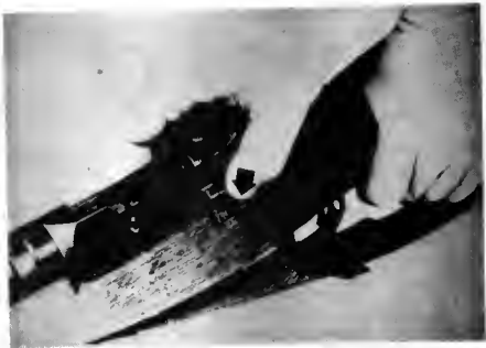
Figure 5. Locking the bolt to the rear
